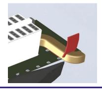
The Simplex A-400M FAS represents the very latest in aerial fire-fighting technology and capability and is ideal for aircraft assigned to multi-mission tasks. The FAS can be installed or removed by a minimal crew in ~90 minutes. The discharge is via gravity only and is fully evacuated in <10 seconds. The retardant exit is via "S" ducts installed in replacement paratrooper doors.
