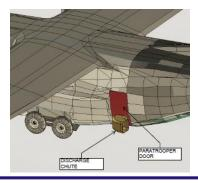
The Simplex C-27J FAS represents the very latest in aerial fire-fighting technology and capability and is ideal for aircraft assigned to multi-mission tasks. The FAS can be installed or removed by a minimal crew in 60-90 minutes. The discharge is via gravity only and is fully evacuated in <7 seconds. The retardant exit is via "S" ducts installed in replacement paratrooper doors.
