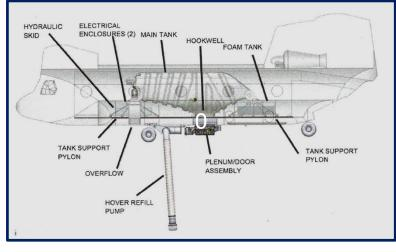
Simplex Aerospace based in Portland, OR, is the world leader in airborne fire-fighting systems. The company has recently completed the development and certification of a unique Fire Attack System for the Boeing CH-47 Chinook heavy lift helicopter for Oregon-based launch customer Columbia Helicopters. This new system comprises a rollon/roll-off internal tank with а capacity of 2,800 US gallons of fire retardant.
